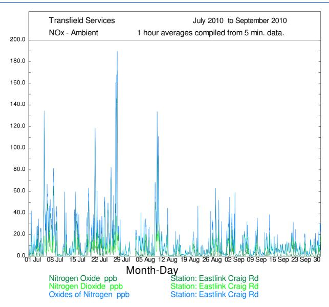
Figure 3: Craig Rd NO, NO<sub>2</sub>, NO<sub>x</sub> 1-hour Averages for July to September 2010
