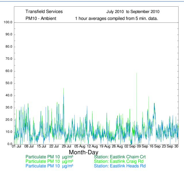
Figure 5: PM<sub>10</sub> 1-hour Averages for July to September 2010
