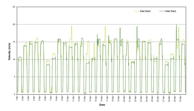
Figure 7: Stack Velocity (1 Hour Average)
