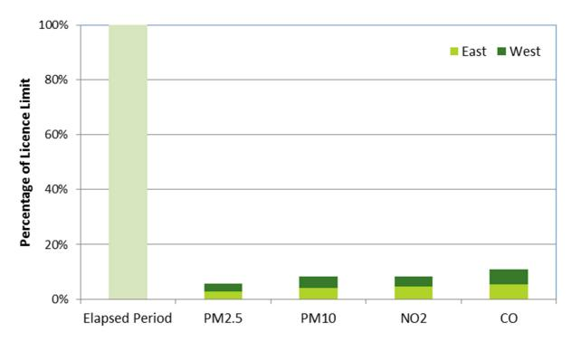
Figure 20: Ventilation Stack Emissions as Percentage of Licence Limit (1/07/2012 - 30/06/2013)
