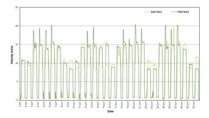
Figure 19: Stack Velocity (1 Hour Average)
