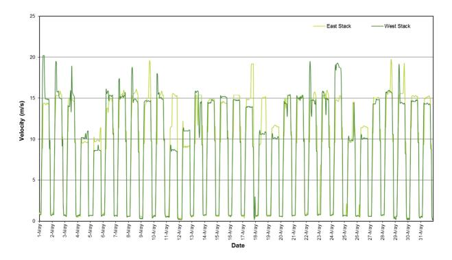
Figure 13: Stack Velocity (1 Hour Average)
