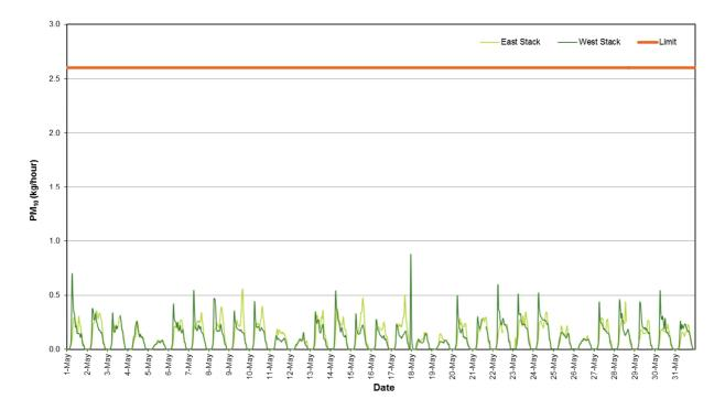
Figure 9: PM<sub>10</sub> Mass Rate (1 Hour Average)
