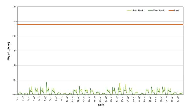
Figure 14: PM<sub>2.5</sub> Mass Rate (1 Hour Average)
