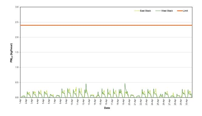
Figure 2: PM<sub>2.5</sub> Mass Rate (1 Hour Average)
