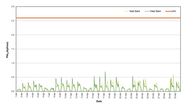
Figure 3: PM<sub>10</sub> Mass Rate (1 Hour Average)
