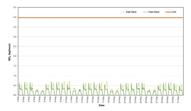
Figure 12: Nitrogen Dioxide Mass Rate (1 Hour Average)
