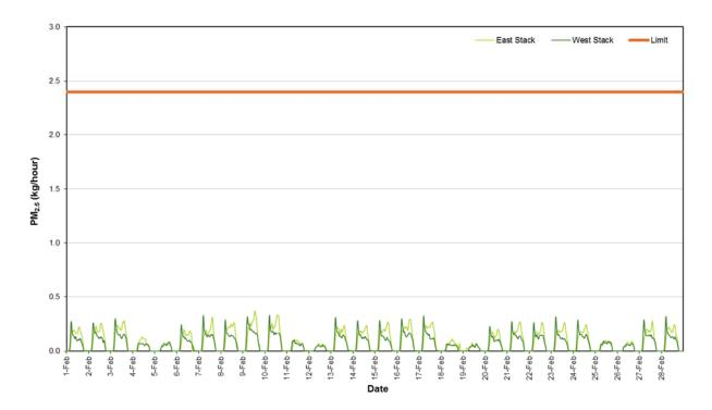
Figure 8: PM<sub>2.5</sub> Mass Rate (1 Hour Average)
