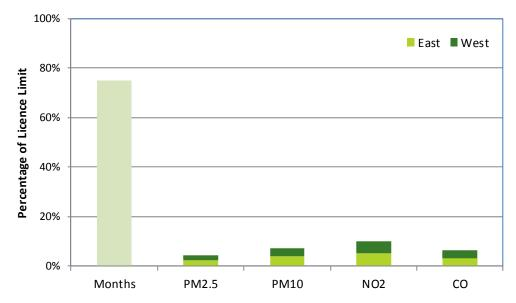
Figure 20: Ventilation Stack Emissions as Percentage of Licence Limit (1/07/2016 – 31/03/2017)
