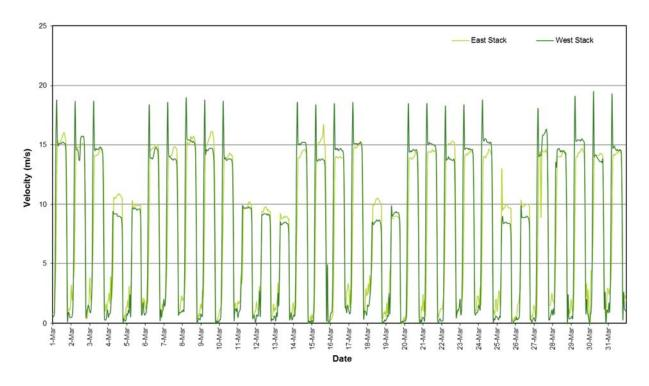
Figure 19: Stack Velocity (1 Hour Average)
