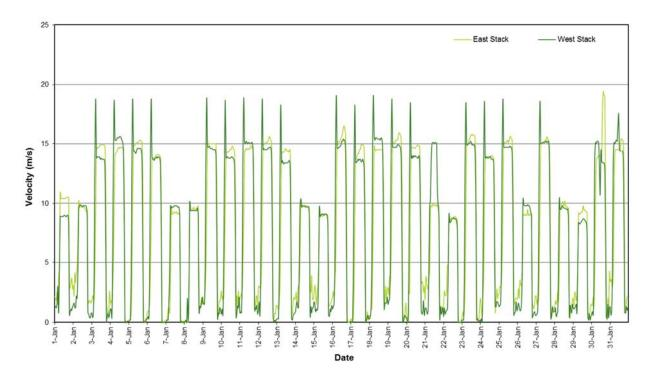
Figure 7: Stack Velocity (1 Hour Average)
