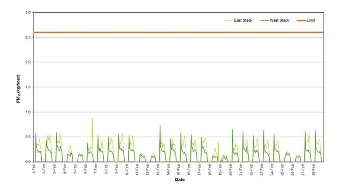
Figure 9: PM<sub>10</sub> Mass Rate (1 Hour Average)
