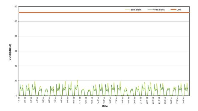
Figure 10: Carbon Monoxide Mass Rate (1 Hour Average)
