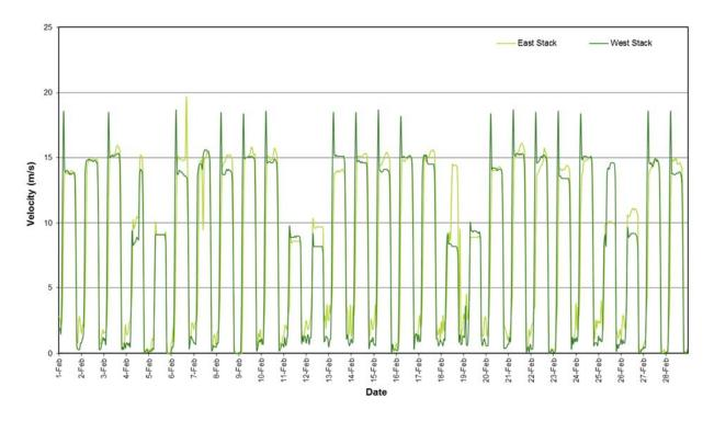
Figure 13: Stack Velocity (1 Hour Average)
