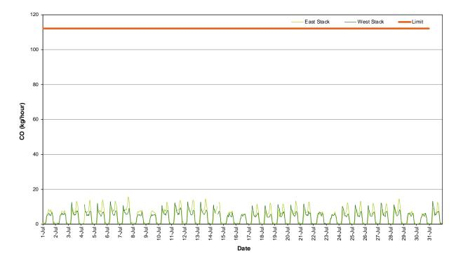
Figure 4: Carbon Monoxide Mass Rate (1 Hour Average)
