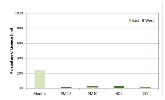
Figure 20: Ventilation Stack Emissions as Percentage of Licence Limit (1/07/2016 - 30/09/2017)
