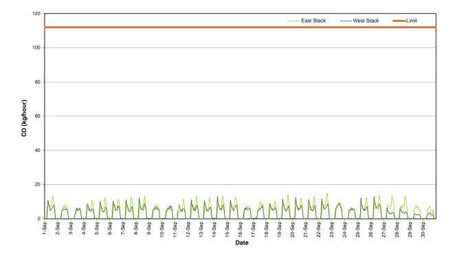
Figure 16: Carbon Monoxide Mass Rate (1 Hour Average)
