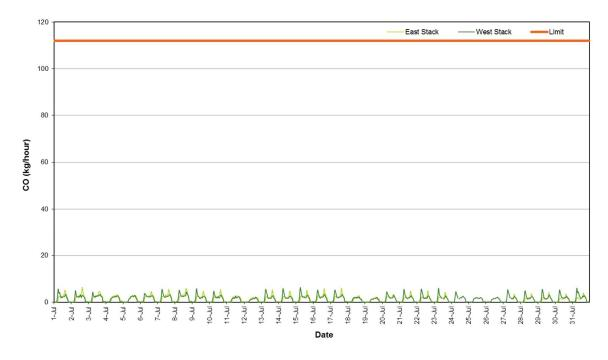
Figure 4: Carbon Monoxide Mass Rate (1 Hour Average)
