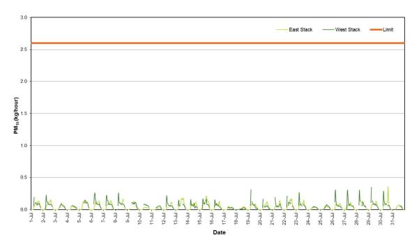
Figure 3: PM<sub>10</sub> Mass Rate (1 Hour Average)
