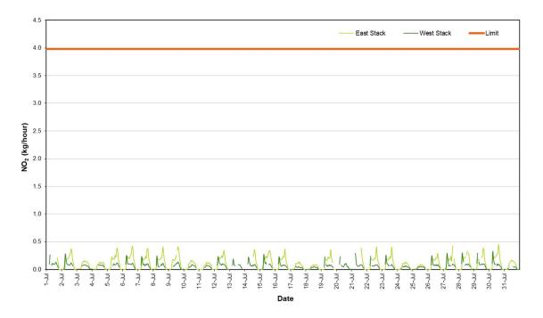
Figure 6: Nitrogen Dioxide Mass Rate (1 Hour Average)
