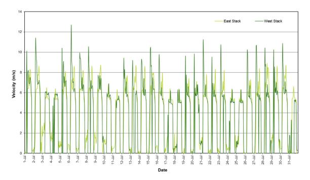
Figure 7: Stack Velocity (1 Hour Average)
